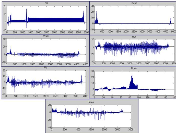
Fig. 2. Plotted accelerometer raw data for different activities
